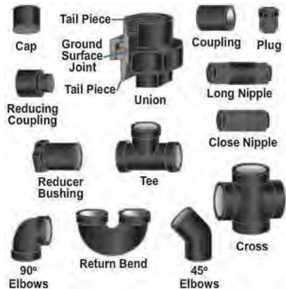
Figure 9-27 – Threaded pipe connectors.
