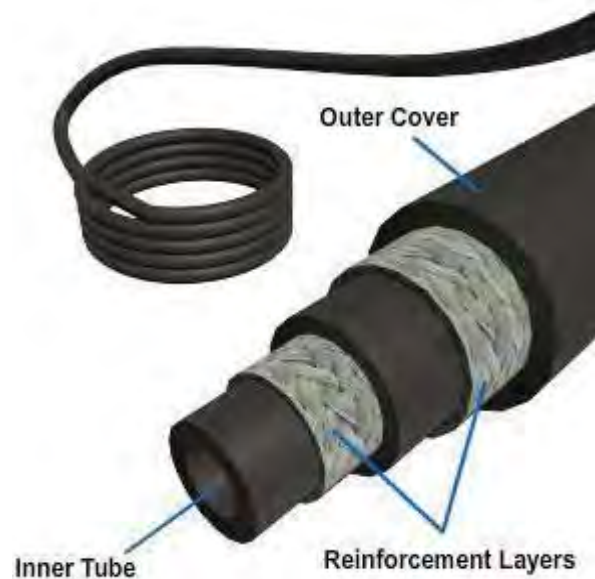
Figure 9-25 – Flexible rubber hose construction.
